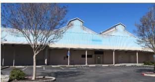
On the north elevation, where a new slightly higher parapet is proposed, both the new parapet and any new construction should remain below the height of the outermost edge of the monitor roofs.
